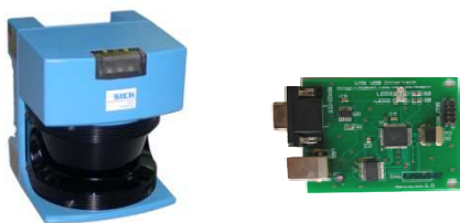
Figure 3. Left) SICK laser scanner. Right) Auxiliary circuit that manages the laser readings and sends them via USB to a PC.
