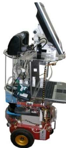
Figure 1. The SANCHO service robot structure. Sancho is constructed upon a commercial mobile platform. Among other capabilities it can project video and interact with users through tactile and voice interfaces.
