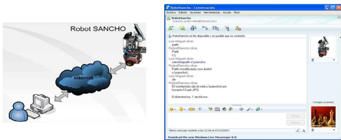
Figure 10. Sancho as a Messenger contact. Left) Sancho connects to Internet as a contact of standard messenger applications. Right) An example of interaction using Windows Messenger Live.
