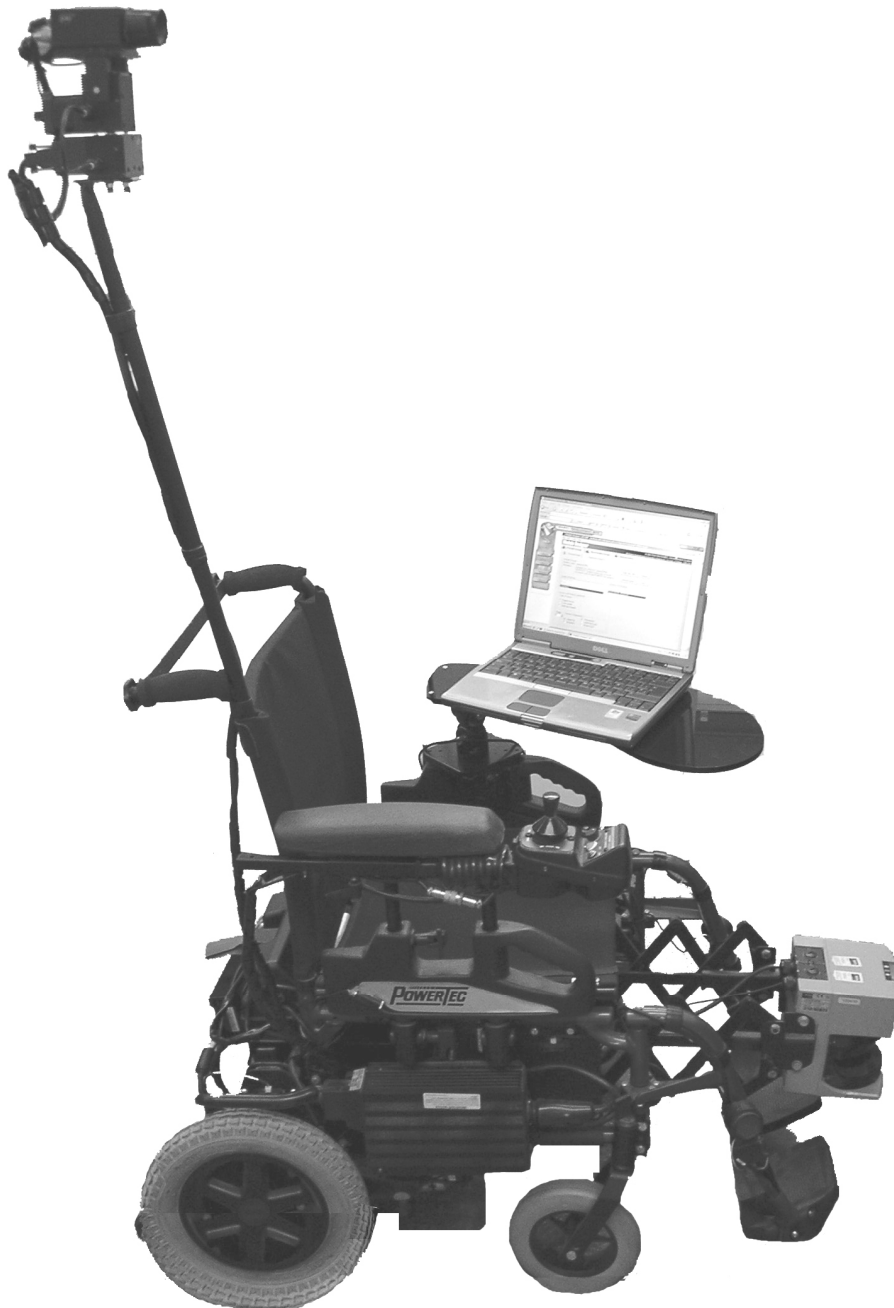
Figure 1 The Robotic Wheelchair SENA. This vehicle is the result of several years of research in the System Engineering and Automation Department at the University of Málaga (Spain).
