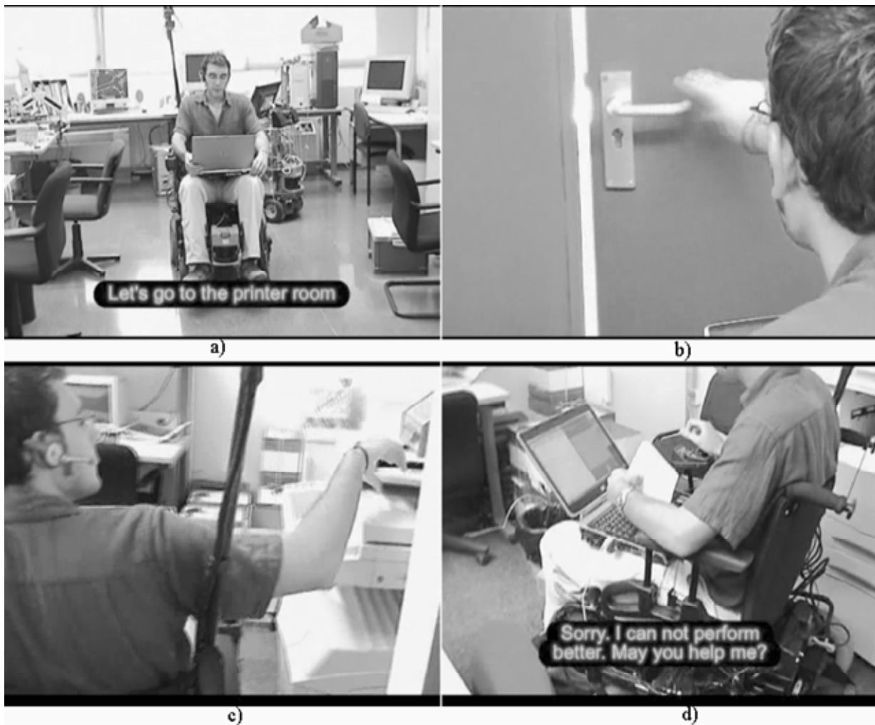
Figure 8. SENA-human integration. When performing within a complex and dynamic scenario, the human help can be required to solve complex situations (b,d). In this sense, SENA and user cooperate: the vehicle provides mobility to the user while she/he manually overcomes the wheelchair limitations.
