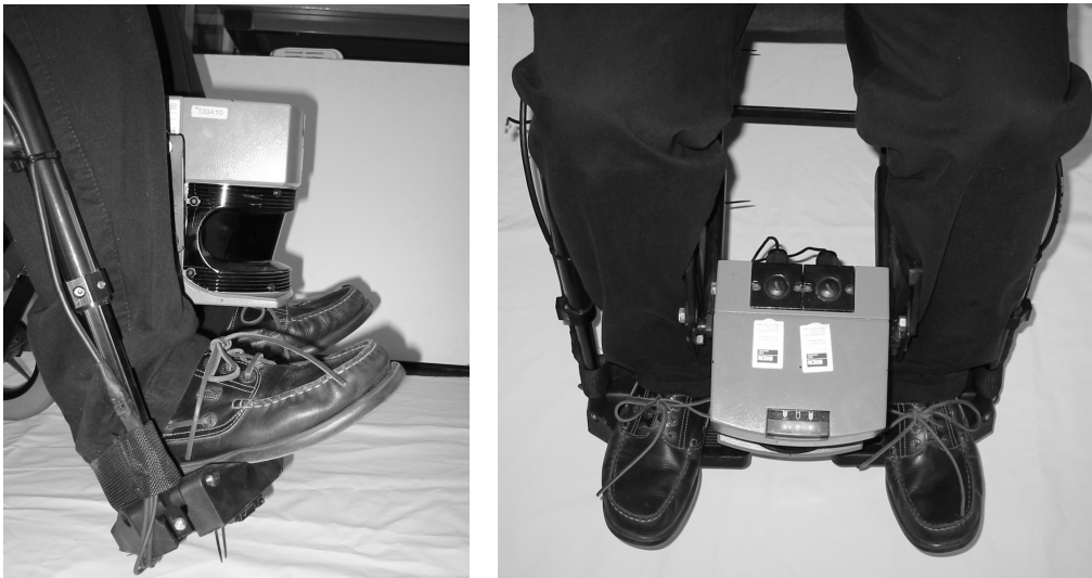
Figure 3. The radial laser scanner provides valuable information from the environment for obstacle avoidance, self-localization, mapping, etc. Its placement in front of the wheelchair permits it to scan with no dead angles and without obstructing the user.
