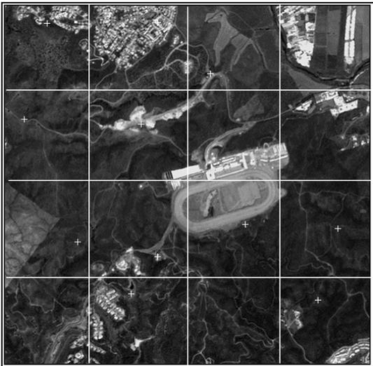
Figure 1. Tessellation of an image and control points detected by the KLT algorithm (marked as +).
