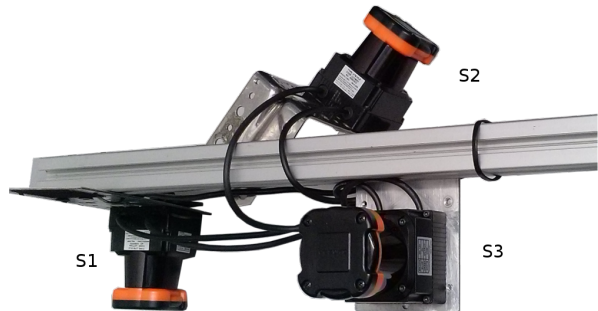
Figure 11: Test LRF rig with three Hokuyo UTM-30LX.
