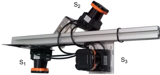
Figure 2.12: Test LRF rig with three Hokuyo UTM-30LX.
