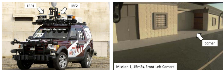
Figure 2.15: MIT’s autonomous vehicle Talos (left), and a snapshot of the corner observed by the lasers 2 and 4 of this vehicle during the 2007 Darpa Urban Challenge (right).
