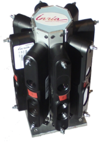
Fig. 5. Omnidirectional RGB-D camera rig.
