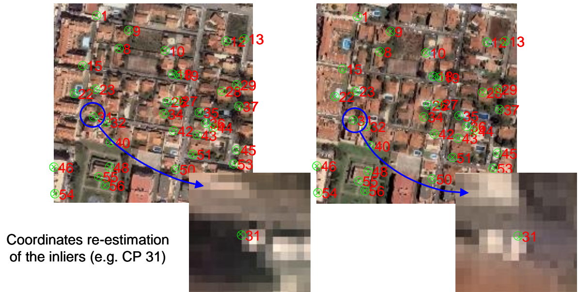
Figure 7: Refinement of the control point pairs detected in two QuickBird images of a typical urban scene: a) robust detection of the outlier matches and b) coordinates re-estimation of the inliers. The enlarged images show, in detail, the actuations described in section 3.2.
