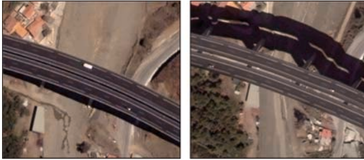
Figure 1. Pair of QuickBird satellite images of the same scene taken from different observation angles. Note the geometric and radiometric differences between both images. Available in colour online.
