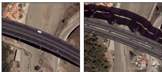
Figure 1: A pair of QuickBird satellite images of the same scene taken from different observation angle. Observe the geometric and radiometric differences between both images.
