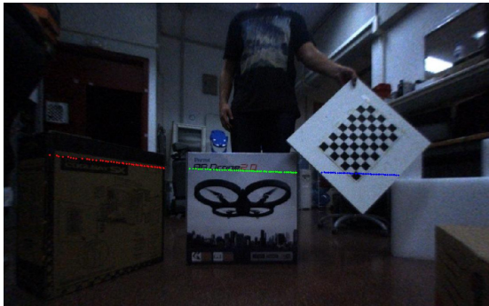
Fig. 8. Projection of the LRF points that belongs to planar surfaces onto the image with the estimated calibration. Our estimation is visually validated as the projection of points fits with the planar objects in the image.
