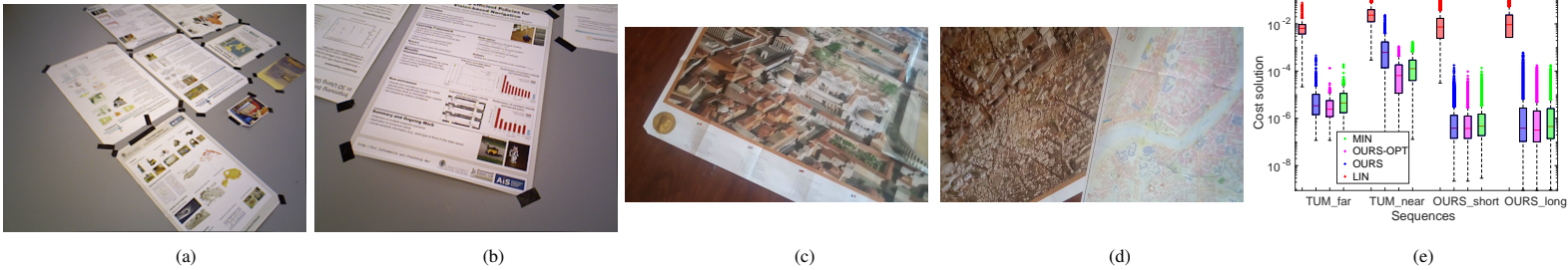
Fig. 6: Figures 6a-6d show images from the real datasets, from left to right: TUM-FAR, TUM-NEAR, OURS-SHORT and OURS-LONG and Figure 6e depicts the cost for the associated essential matrix attained by the different solvers for the same sequences, including those certified as optimal OURS-OPT.
