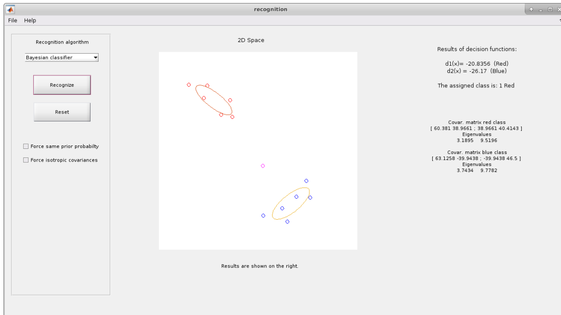
Figure 7. Recognition GUI illustrating the recognition of an object instance (magenta point) as an object of the red class.
