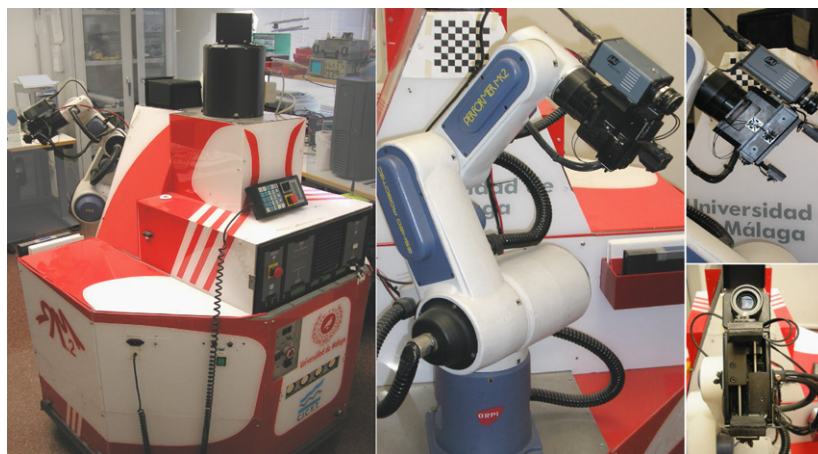
Fig. 3. Different views of the performer MK2 industrial manipulator arm. It is mounted on the RAM-2 mobile robot (as well as its controller-B), although it can also be used independently on the platform. In the figure you can see the main features and components of the robot, including the camera and collision sensors in the gripper.
