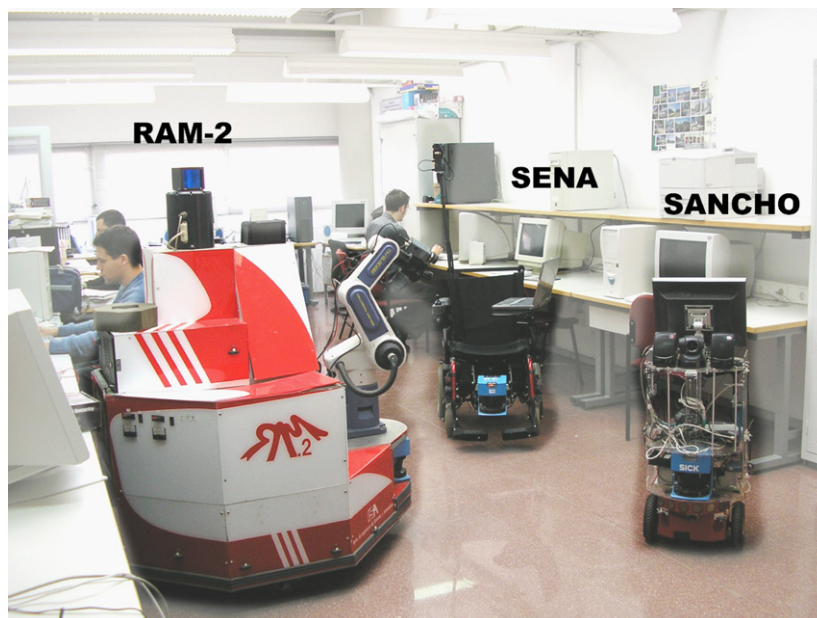
Fig. 2. A view of three mobile robots in our research laboratory. From left to right: our mobile manipulator RAM-2, our assistant robotic wheelchair SENA, and our service robot SANCHO.
