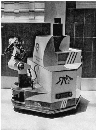
Fig. 9. The Explorer laser range scanner mounted on the RAM-2 mobile robot.
