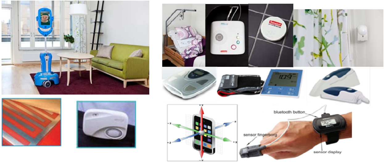
Fig. 6 The Giraff robot in the test apartment. Examples of Tunstall sensors: first line from left to right: Bed/Chair Occupancy Sensor - Gateway collecting sensor data - Flood detector - Fast PIR (Movement Detector); second line from right Enuresis Sensor - Fall Detector - Fast PIR (Movement Detector). Sensors from IntelliCare: in the middle from left to right: scale, blood and glucose sensor, thermometer, portable pulse and oxygen sensor.
