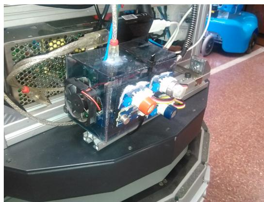
Figure 6: Picture of the e-nose used in the experiments for the detection (and posterior classification) of acetone and ethanol. The e-nose is composed of an array of 10 MOX gas sensors with overlapping selectivity and detection range.
