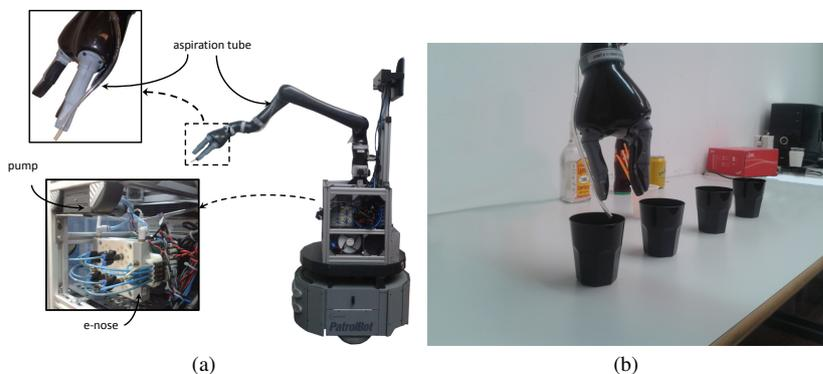
Fig. 8: (a) The robotic arm used in the third experiment mounted over a mobile platform, and a detailed view of the attached e-nose aspiration. (b) Picture of the proposed setup for the third experiment. Each of the black plastic vessels contains a different substance.
