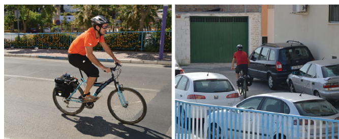
Fig. 4. Pictures taken during the data collection carried out in Coin (Málaga) for the monitoring of waste related odors. The bike was equipped with an e-nose comprising an array of 7 MOX gas sensors and a GPS for proper localization of the measurements.
