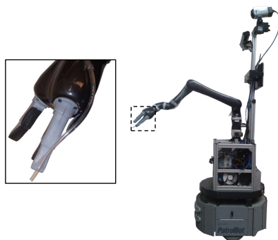
Figure C.4: The JACO robotic arm mounted on a mobile platform, and a detailed view of the attached e-nose aspiration.
