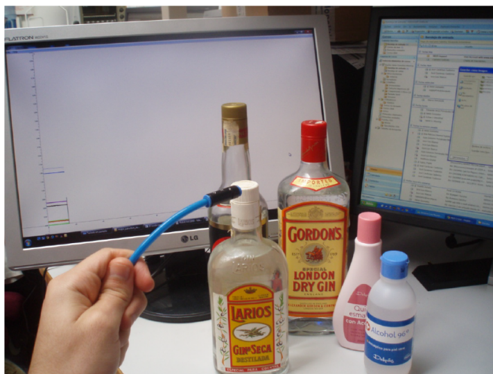
Figure C.1: Snapshot during the collection of the first presented data-set. It can be seen the e-nose aspiration (blue thin tube) and containers of different target odors.
