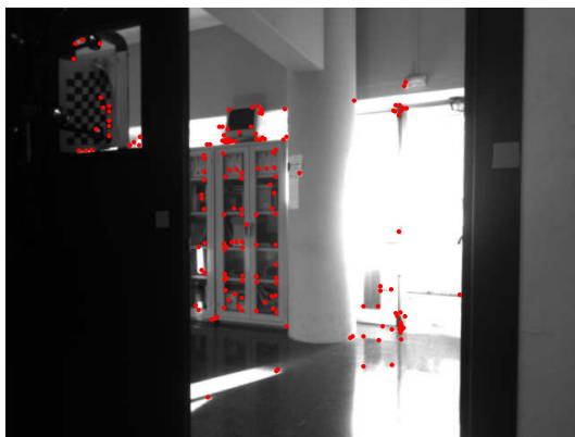
Figure 4.10: An example of ORB features detected in a real image.
