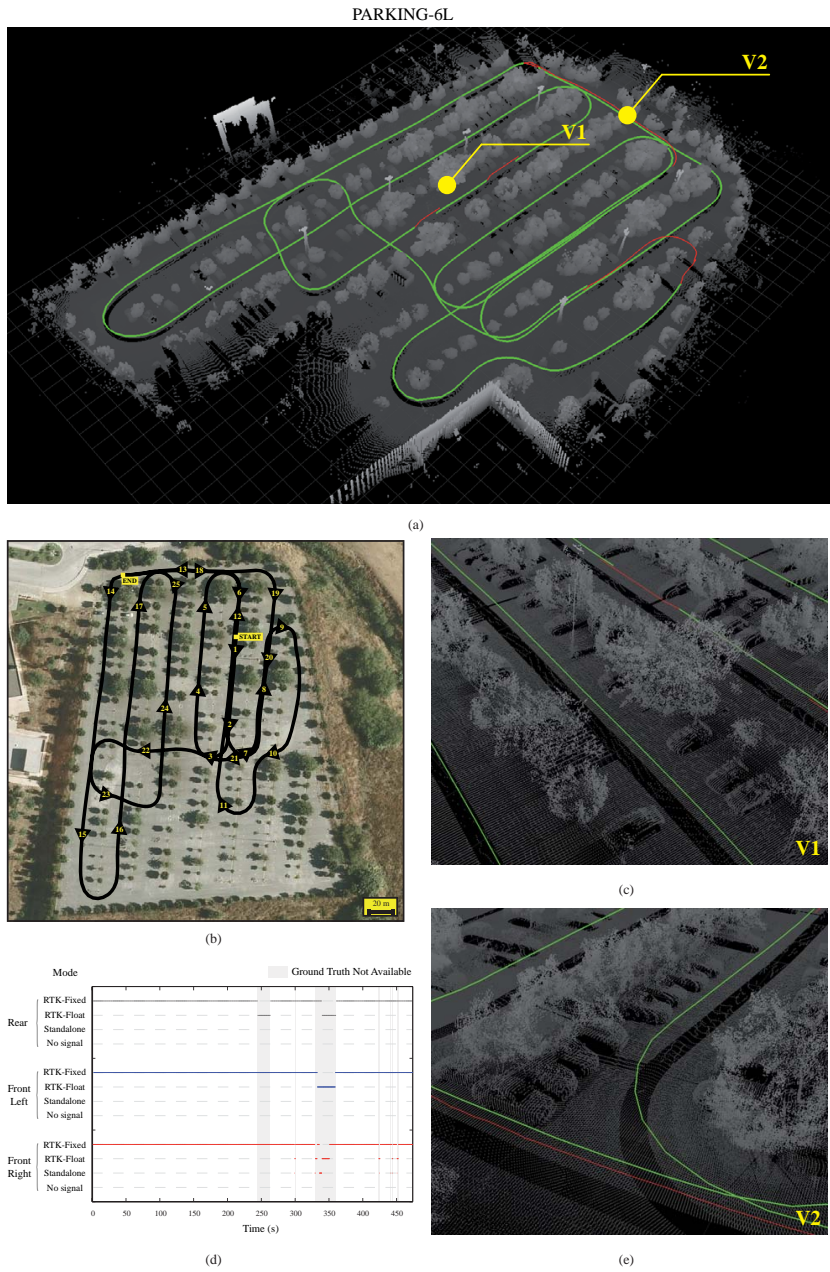
Figure 5.9: PARKING-6L dataset. (a) 3D projected points for the lateral laser scanners and vehicle path. (c,e) Zoom of zones V1 and V2. (b) Top-view of the vehicle path and (d) status (modes) of the 3 GPS devices during the experiment.
