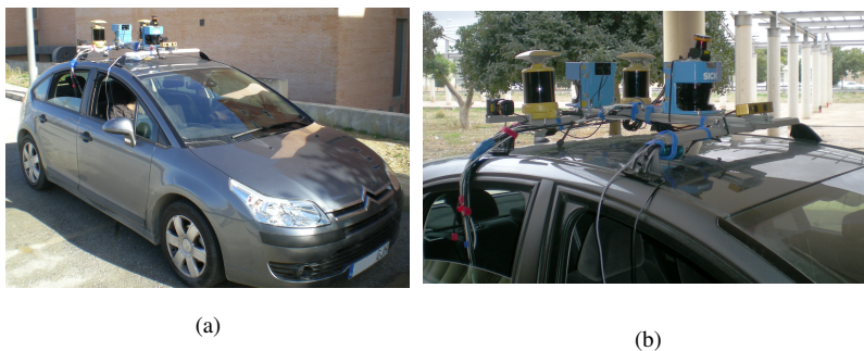
Figure 5.22: The instrumented vehicle employed for collecting the dataset: (a) general view and (b) close-up of the sensors.
