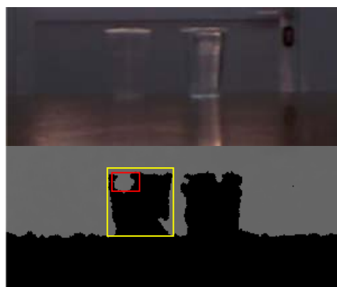
Figure 6. Up, RGB image of part of the scene. Bottom, range image. Black pixels represent lost measures. The red rectangle marks a sample area where Kinect returns the depth of the door placed behind the plastic cup.
