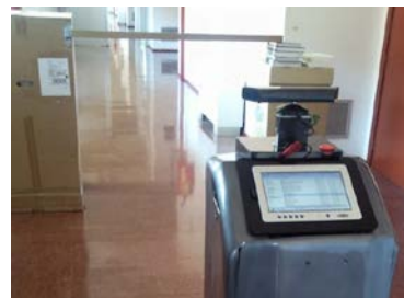
Figure 10. Test process for detecting thin objects. In this case the thickness of the object was 4 cm.
