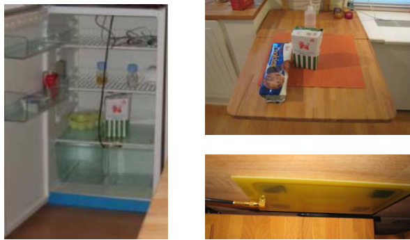
Figure 9: Left: the fridge used in our experiment, equipped with a door opening mechanism and an RFID tag reader. Right: the RFID tagged milk box on the kitchen table, equipped with a second RFID tag reader.
