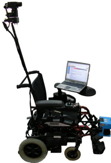
Figure 8. The robotic wheelchair SENA. It is based on a commercial powered wheelchair which has been endowed with several sensors and devices. The SW architecture runs on the user's laptop, who can still use it for her/his work.
