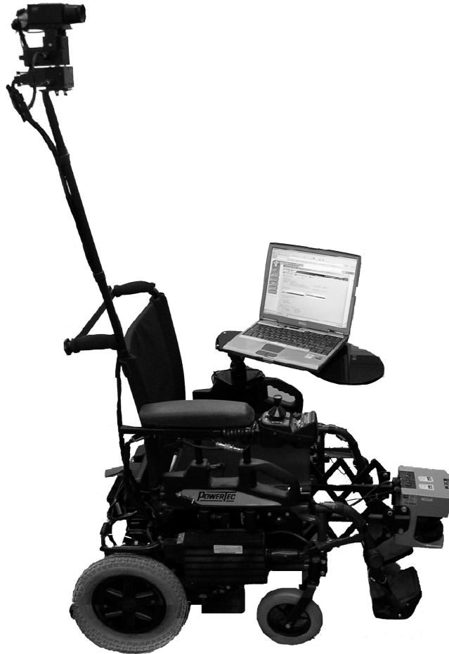
Fig. 1. The robotic wheelchair SENA. It is based on a commercial electric wheelchair which has been endowed with several sensors (infrared, laser, and a CCD camera). Wheelchair motors as well as sensors are managed by a microcontroller communicated to a laptop computer via USB.
