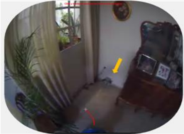
Figure 3. Image provided by the Pilot application taken during a manual docking operation. The recharging station is marked with a yellow arrow for illustrative purposes.
