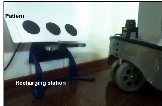
Figure 4. Detail of the recharging station of the Giraff robot. The pattern used for localizing the docking station is placed centered on it.
