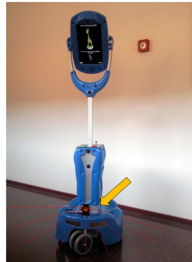
Figure 8. The Giraff telepresence robot. The Hokuyo sensor (marked with an arrow) is placed on the base where it scans 240^\circ in a plane parallel to the ground. Some range scans have been recreated in the figure for illustrative purposes.
