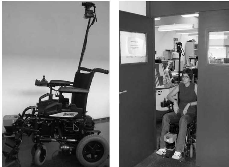
Figure 4. Two views of the SENA robotic wheelchair in which we have evaluated our human-robot integration architecture.
