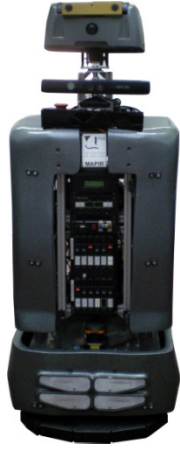
Figure 7. Mobile robot SANCHO, equipped with 2 Hokuyo laser scanners and a Kinect sensor for obstacle avoidance.
