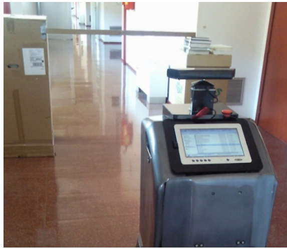
Figure 3. Experiment setup to test the “visual acuity” of Kinect for detecting small obstacle. In this particular case, the obstacle is a horizontal stick with a thickness of 4 cm.
